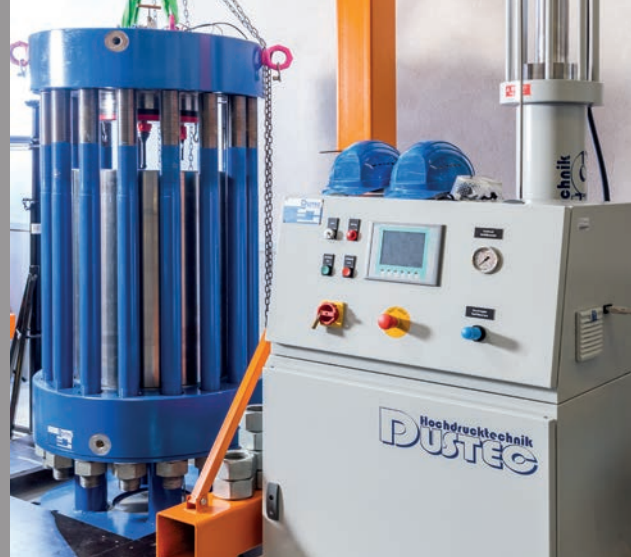
This pressure chamber can generate a pressure of 1200 bar corresponding to 12 000 m ocean depth.
