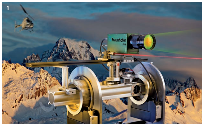
1 Laser-Based Helicopter Obstacle Warning.
