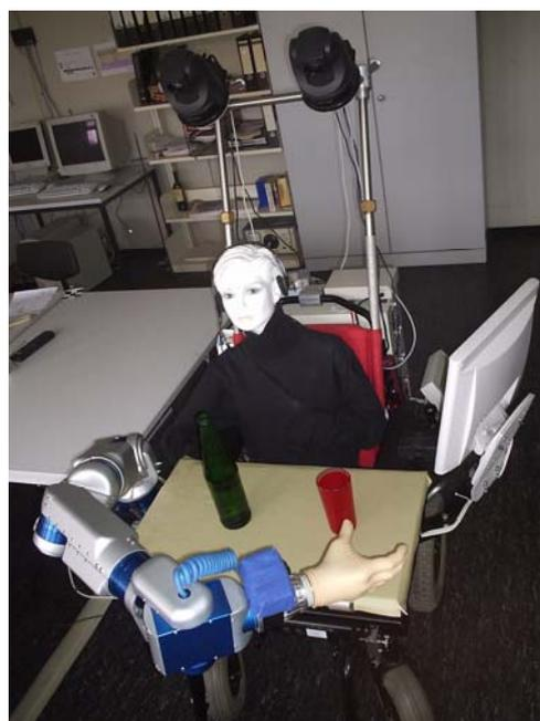
*Figure 1: Rehabilitation robotic system FRIEND II*
