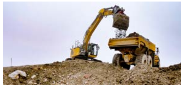
Autonomous loading by an excavator in a landfill. (Photo: Fraunhofer IOSB)
