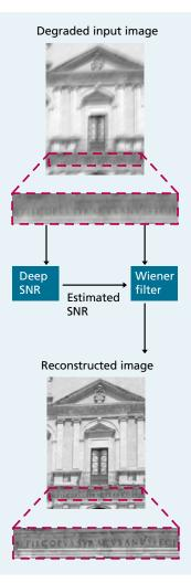
Example application of Deep SNR-based Wiener filtering of a degraded input image from [2].
