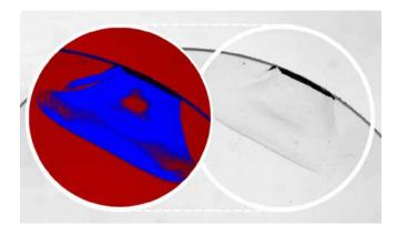
The advantage of light field illumination (left) in direct comparison to traditional bright field illumination of the same specimen.
