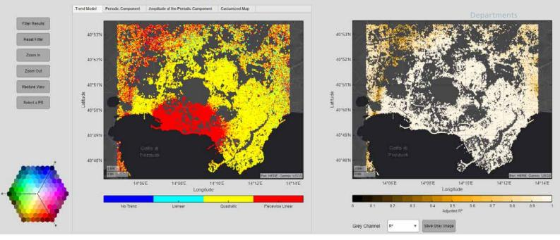
Visualization of PSDefoPAT results generated from displacement time series by the European Ground Motion Service.
