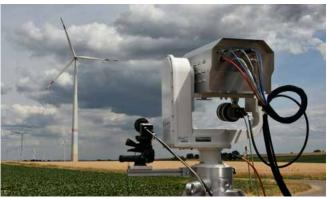
Laser Doppler vibrometer for taking measurements on moving objects.
