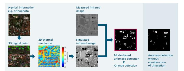
Schematic representation of simulation-assisted detection of human activity in IR images.
