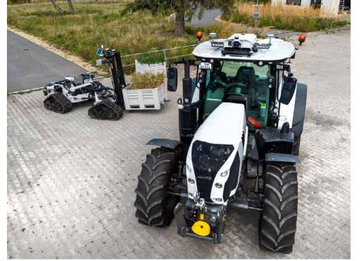
Retrofitting mobile machines with environmental sensing capabilities: the Environment Perception Kit in use.
