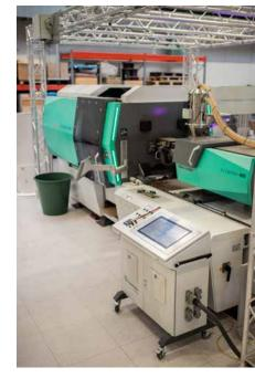
INArice traverse module equipped with sensors, monitoring an injection molding machine, as an example of contactless data acquisition using optical sensors.
