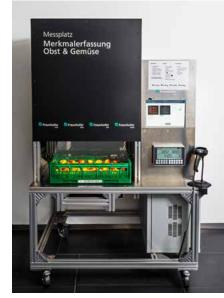
The Al-based analysis of standard fruit crates is performed directly on the multisensory scanner.
