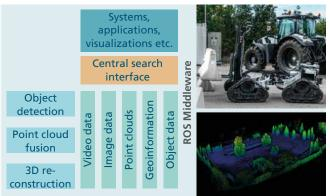
Overview of the components of the MUSAL ecosystem, sample autonomous mobile systems, and generated point cloud data.
