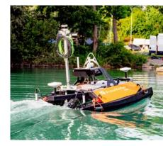
TAPS — autonomous sensor carrier.
